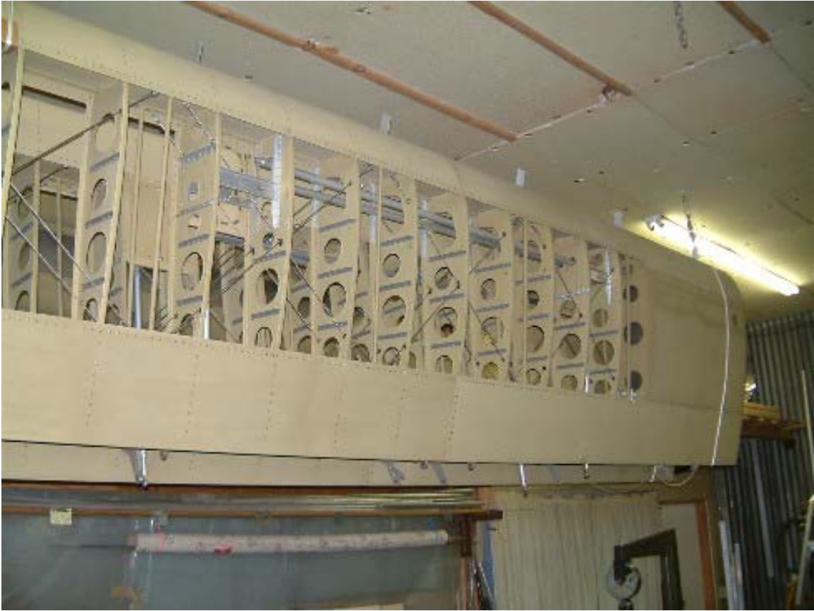
WING SECTIONS to be covered with fabric.
