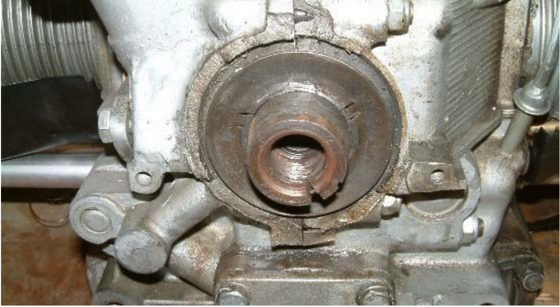
The crank after the hub failure
