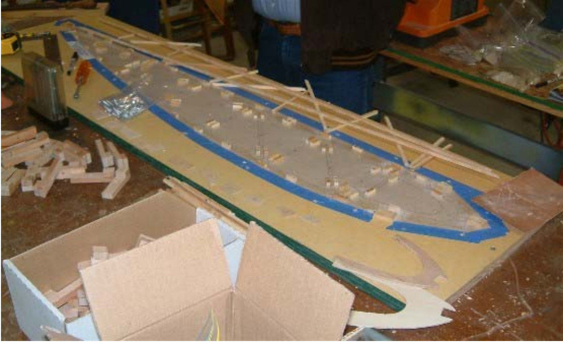
Jig for the new ribs and the pieces for the demonstration.
