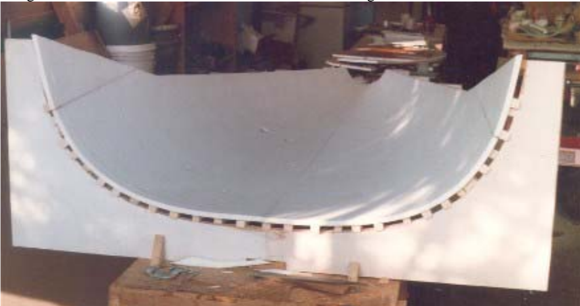
MOLD FOR REAR DECK READY FOR GLASS INSIDE.
