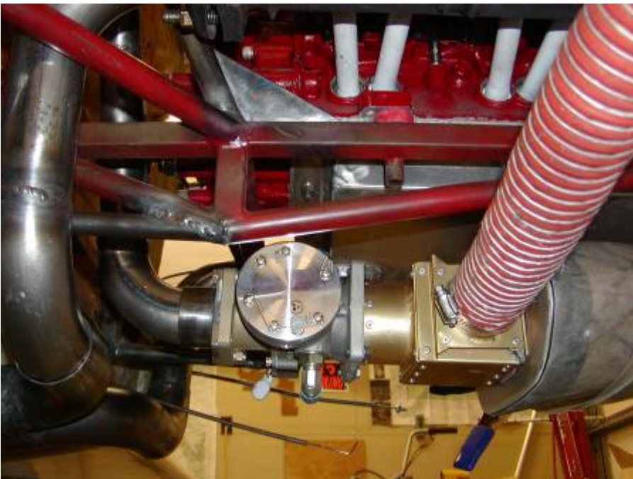
Preliminary assembly shot with Ellison, carburetor heat box, and filter air-box.
