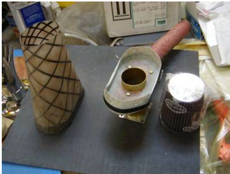
A custom air-box for the K&N cone filter to sit in. I plan on a velocity stack behind the prop feeding the sealed air-box
